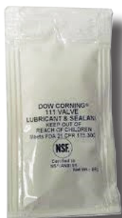
Dow Corning 111 Valve Lube Used to lubricate PE Pipe before insertion into ID Seal® Con-Stab Fittings Catalog # 34-7287-00
