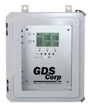
The GDS Corp *Protector4* System Controller is designed to provide power for and monitor signals from up to four industry-standard 4-20mA devices, including all GDS Corp gas monitors, sample draw monitors and process monitors.
