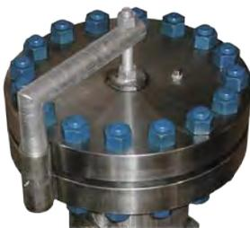
Removable perforated 304SS Safety Screen sits under (down-stream of) filter element(s) to guard against lost pens, stray coins, and other undesirable items at time of filter element change out.
