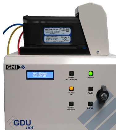
Figure 91 : Station d'étalonnage GDUnet
