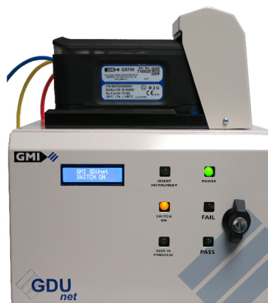
Figure 82 : Station d'étalonnage GDUnet
