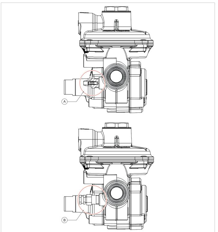
Fig. 4.6. Pressure outlets
