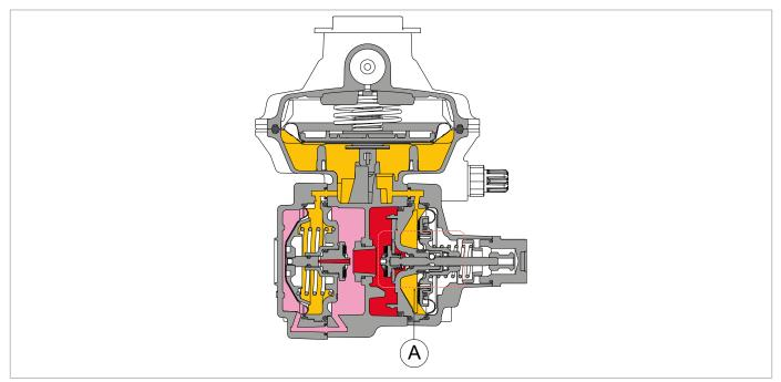
Fig. 4.3. Slam-shut valve for maximum pressure
