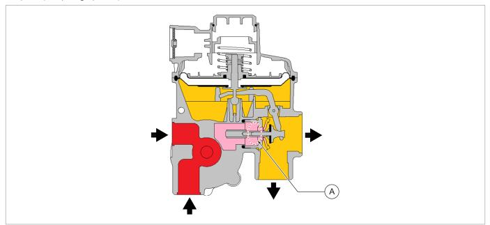
Fig. 4.4. Excess flow safety device
