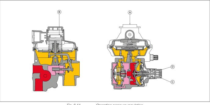
Fig. 6.11. Operating pressure regulation
