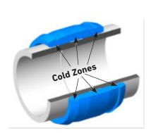
Equally as important as the heating phase of the fusion cycle, the cooling phase is a defined part of the electrofusion process. Because polyethylene is a thermoplastic, the material softens when heated and is therefore vulnerable to stresses from external forces such as the weight of the pipeline and bending
