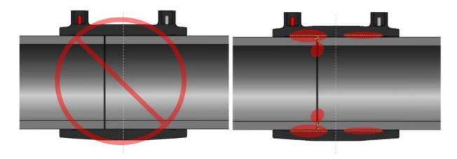
Mis-Cut – Another potential error that can cause loss of melt containment is the lack of a square cut on the pipe ends. While it is not necessary, nor practical, that the pipe ends must be cut to exactly 90 degrees, care should be taken to keep the cut as square as possible. Cold zone lengths are designed to accommodate some degree of mis-cut on the pipe ends and still ensure full coverage of the heating wires and sufficient cold zone contact to contain melt flow.
