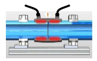
forces from pipe curvature or misalignment while it is still hot. Fittings must be held stationary and in alignment by clamps during the fusion and cooling process to protect against inadvertent disturbance of the molten PE until the assembly has cooled and regained its material strength.
