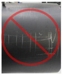
Poor scrape: markings not removed
