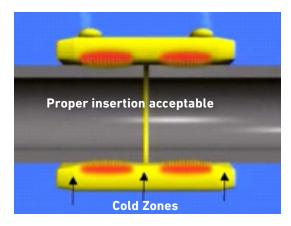
A pipe end that is not inserted beyond the innermost heating wire is commonly referred to as being "short-stabbed" and is the result of an assembly error.
