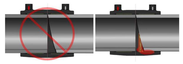
Pipe End Cutting Procedure: To ensure that the pipe ends can be correctly inserted into the center of the electrofusion coupling, do the following:
