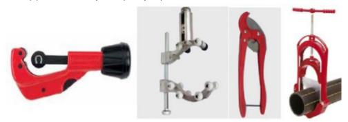
For smaller pipe or tubing sizes, cutters made for this purpose work well. For larger pipe sizes that are cut by hand, make a guide mark around the pipe that can be followed with the cutting tool. To accomplish this, a wrap-around strap can be used to ensure a straight mark. Chainsaws or reciprocating saws may be necessary for large diameter pipes. If using a chainsaw, do not use chain oil.
