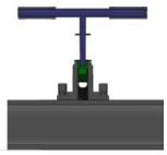
5. Remove tapping tool. Lubricate cap and chimney O-rings if needed and replace cap. Tighten cap hand tight only, do not use wrenches. Check for leaks per normal procedures.
