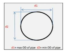
Figure 3 Diameter measurement diagram
