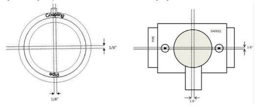
Cut FET specimens approximately 1/16 to 1/26 inches wide from each fusion or joint half. A minimum of four FET strips shall be cut from each end of the socket and from the saddle spaced approximately 90° apart.
