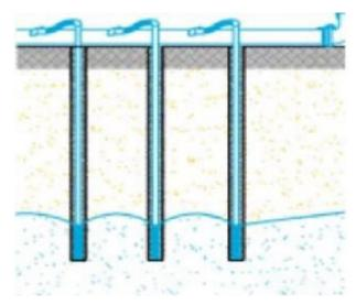
Figure 2 Well point dewatering system
