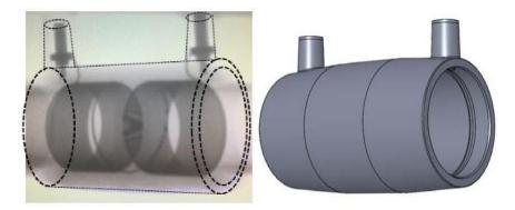
X-ray perspective of heating coil mechanism
