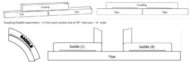
Saddle specimen – 4 total, 2 radial from each side, 2 axial from each side at  $90^{\circ}$  intervals  $\times$  1/8" wide
