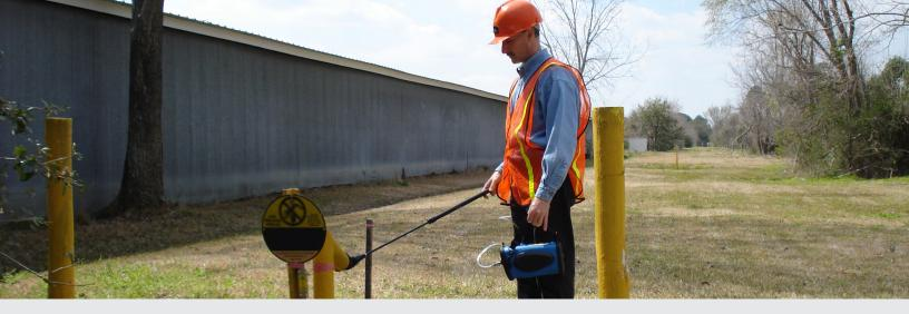
The Detecto Pak-Infrared (DP-IR) is an extremely sensitive, advanced leak detector capable of detecting methane without false alarming on other gases. The DP-IR is the latest generation of leak survey instruments from Heath that will greatly improve the productivity and safety of a walking/ mobile survey because of high sensitivity and fast response. It is also an effective tool for Method 21 emissions leak detection.
