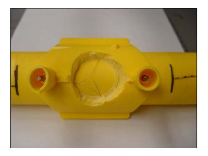
Figure 7. Impact Test on electro-fused saddle tee to ASTM F905.
