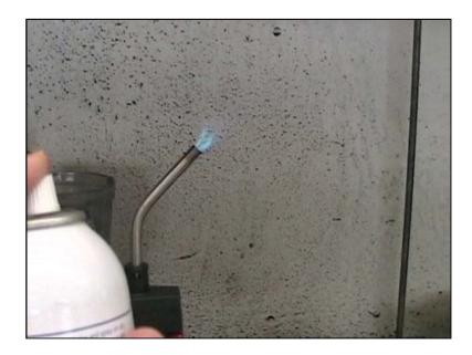
Figure 6. Flammability Test. Note that the flame does not increase when sprayed with IGT static suppressor.
