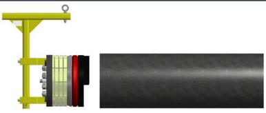
For added safety, use an approved installation device such as TPLIFT-1024 to install the test plug (reference instructions, DC2590)
