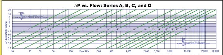
Use the chart above to access the init.  $\Delta P$  vs. flow for series A, B, C,  $\phi$ : D air intakes. Be aware that the maximum practical flow through a filter housing, like other piping, is limited primarily by the cross sectional area of the connection. Compare the connection size shown
