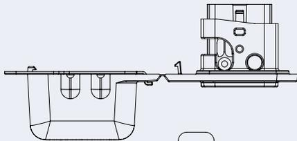
4. Place unstripped tap conductor into side B (see image in step 2). Insert conductor until visible against stop on opposite side.
