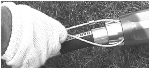
until it comes out the other side. Keep pushing it through until the swaged stop sleeve is almost touching the tailpiece extension. Slide the fused, straight end of the cable through the captive wire rope clip. Slide the wire rope clip towards the tailpiece extension until it is near the swaged stop sleeve and tighten the two nuts on the wire rope clip with a 5/16" wrench. The
