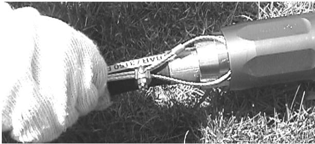
cable to be pulled may now be attached to the loop at the other end of the pulling cable.
