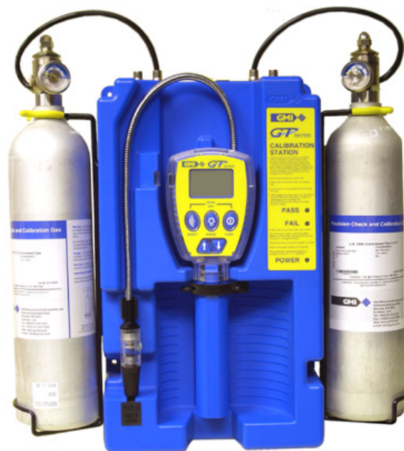
Fig. 1 GT series instrument located in (Mixed Gases) Calibration Station
