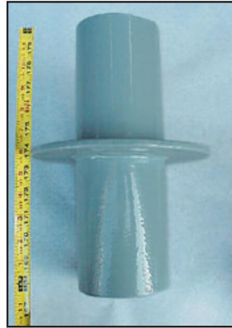
Figure 1: Gal-vo-plast<sup>®</sup> Wall Sleeve submitted for testing
