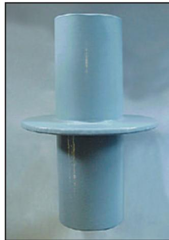
Figure 3: Gal-vo-plast<sup>®</sup> Wall Sleeve after 500 hours of exposure
