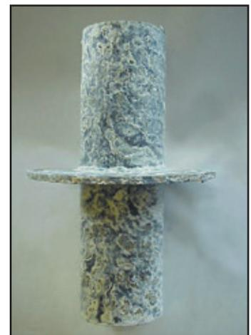
Figure 4: Galvanized Wall Sleeve after 500 hours of exposure
