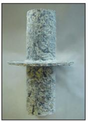
Figure 3: Gal-vo-plast<sup>®</sup> Wall Sleeve after 500 hours of exposure
