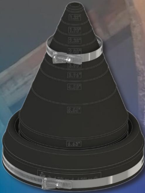
APS manufactures full, molded, conical End Seals with easy to read size indicators for versatile installation on a variety of carrier sizes. Each End Seal comes with a pair of quick adjust Stainless Steel band straps that cover all sizes within the range, so no custom-made items are needed. The End Seals are manufactured from 1/8" thick durable, chemical resistant EPDM rubber.
