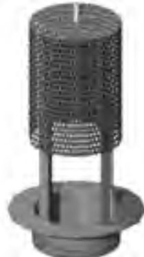
Removable perforated 304SS Safety Screen sits under (down-stream of) filter element(s) to guard against lost pens, stray coins, and other undesirable items at time of filter element change out.
