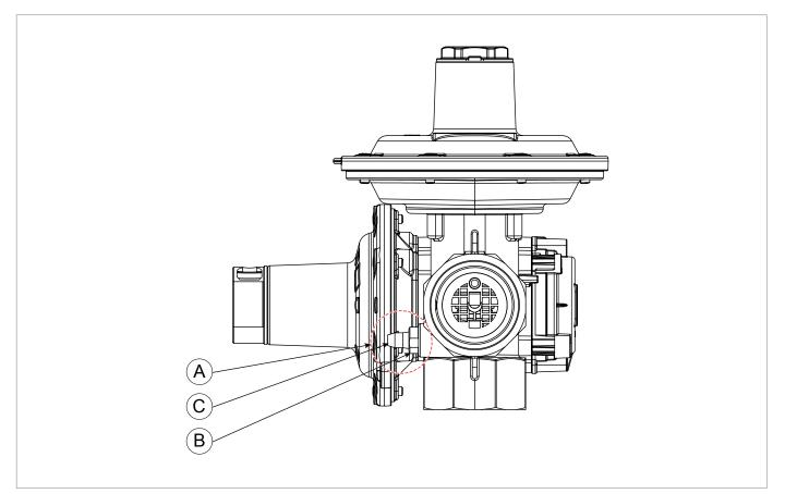
Fig. 4.6. Standard pressure outlet use
