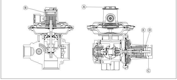
Fig. 6.10. Operating pressure regulation
