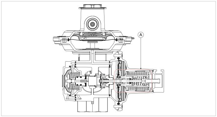
Fig. 4.3. Slam-shut valve for minimum and maximum pressure
