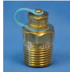
Product: #700 Core: Neoprene Thread: 1/2" NPT Length: 1 1/2"
