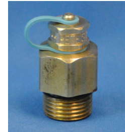
Product: #750 Core: Neoprene with Buna-N O-Ring Sealant Thread: 3/4" - 16 NPT Length: 1 1/2"
