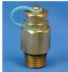
Product: #562 Core: Neoprene with Buna-N O-Ring Sealant Thread: 9/16" NPT Length: 1 1/2"
