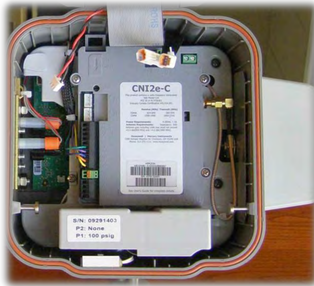
Figure 5. The EC 350's internal digital cellular radio sends audit trail and diagnostic information to the data collection system.
