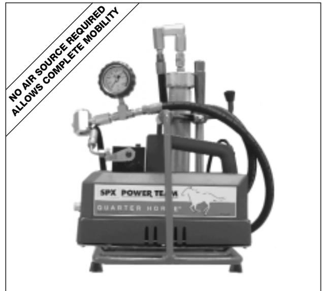
The easy to operate Val-Tex QS-2200A is a fast, compact, rugged lubrication unit. Run by a rechargeable battery powered hydraulic pump, the QS-2200A gives you complete mobility and eliminates the need for an air supply. It is suitable for use with J size lube sealant sticks, Lube Packs, cartridges, and Valve Flush.
