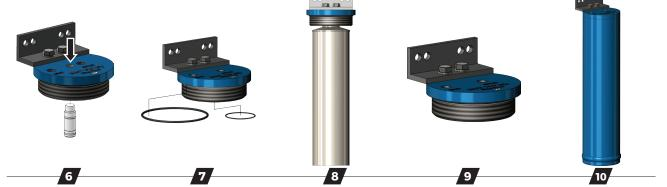
If the filter dryer is equipped with the optional moisture indicator and the moisture indicator has changed from blue to pink, the moisture indicator needs to be replaced. From the top of the top cap, push the moisture indicator out. Install a new moisture indicator with a new O-ring in its place.
