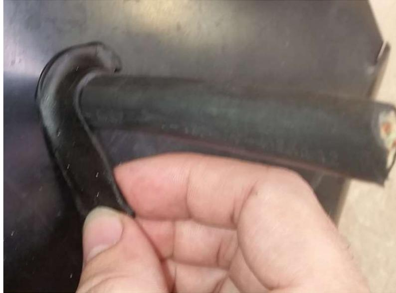
10. Gently Press mastic in to make it stick to both surfaces. The mastic is extremely sticky and will not require a large force to be set in place.
