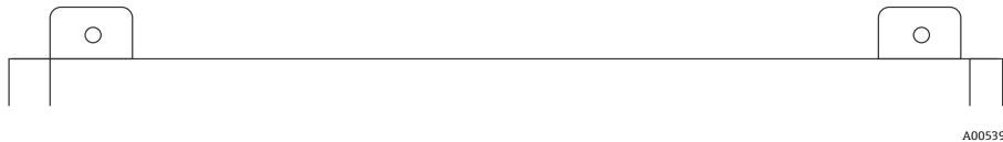
Figure 14. Top mounting tabs of enclosure
