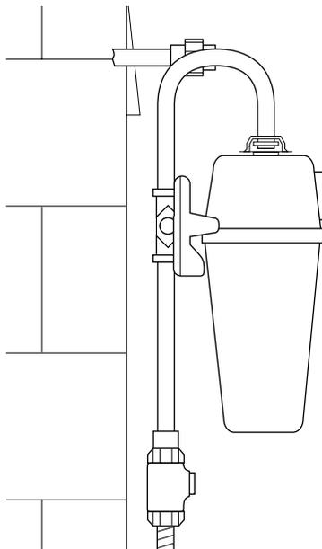
Complete meter installation side inlet – side outlet low pressure
