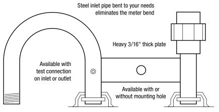
Available with a variety of outlets including insulating unions — positioned side, top or rear to meet house piping
