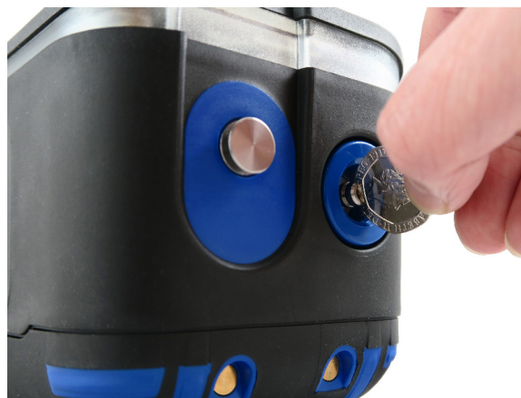
Figure 70: Inlet Nozzle Removal
