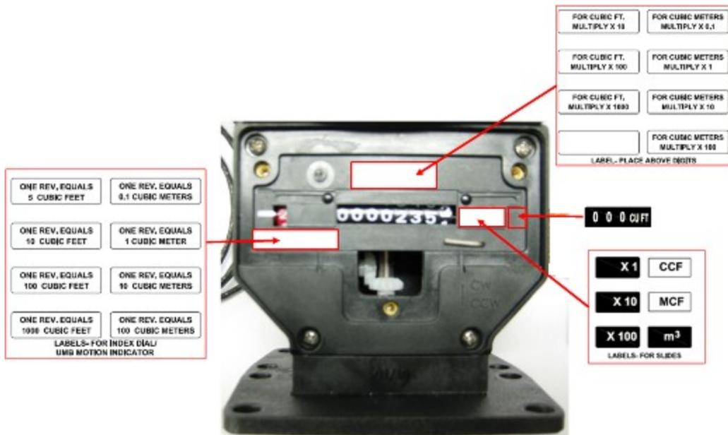
The following image illustrates the labels applied to the UMB, slides, and rivets.
