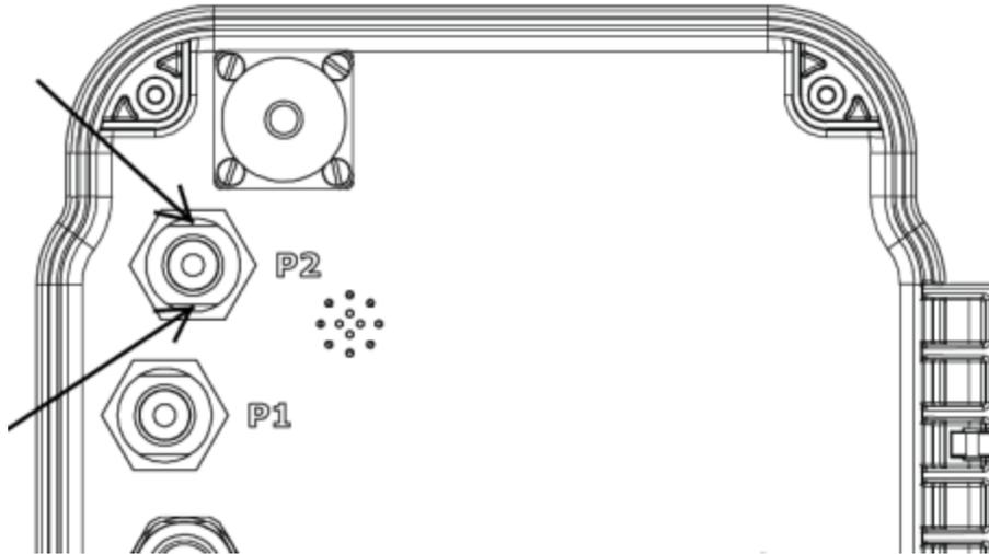
**Warning:** To avoid explosion, it is extremely important to ensure the pressure transducer is capable of handling the pressure in the gas line. Check item entry 137 (user units) or item entry 25(Psi) on the EC350 for maximum pressure transducer information before applying live gas pressure to the EC350.
