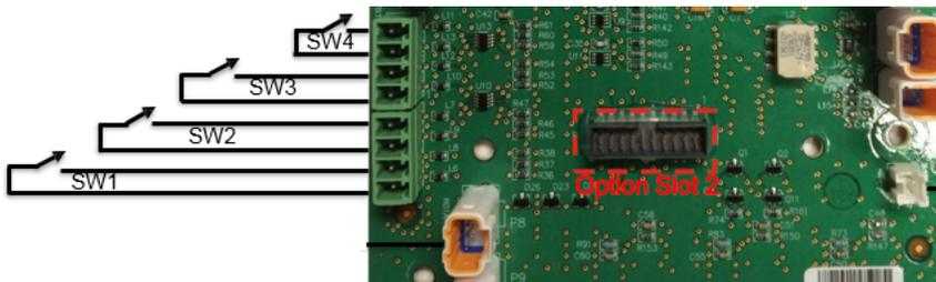
**Note:** If the user wants to use SW3 and SW4 for reverse flow, the digital switch input alarms (i762 & i763) must be disabled.
