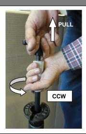
1. Install the Inserter tool on the Lockout Plug by pulling the black T-handle back, and turning the aluminum handle counter-clockwise (CCW) until it becomes hard to turn. Ensure it is installed tight!
