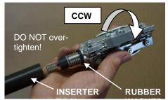
1. While pulling the <u>black</u> T-handle back, insert the Lockout Plug into the Inserter tool as shown and rotate it counter-clock-wise (CCW) until the rubber washer JUST contacts the Inserter tool.
