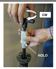
2. While holding the aluminum handle, turn the black T-handle clockwise (CW) to expand the Lockout Plug in the opening. Continue until the Lock-out Plug can no longer be moved up or down.
