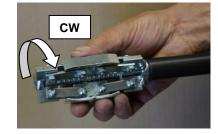
3. While pulling the black T-handle back, unscrew the Lock-out Plug from the Inserter tool by turning it clockwise (CW).
