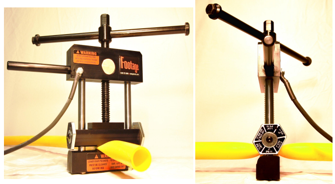
Place tool centrally on pipe & at 90° to pipe
