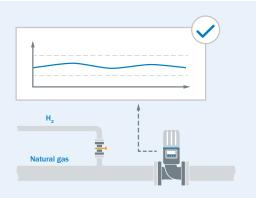
While commissioning the FLOWSIC500, the current gas composition and a permissible deviation can be configured via the Gas Quality Indicator (GQI) in FLOWgate<sup>TM</sup>. The gas quality is constantly monitored.
