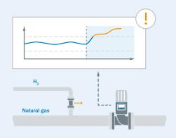
If the gas composition changes due to the incorporation of other gas types, e.g. hydrogen, the operator receives a status notification as soon as the GQI exceeds the configured permissible deviation. Any changes in gas quality can thereby be detected.
