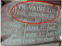
Nameplate: This information is usually found on the nameplate or on the body casting.
