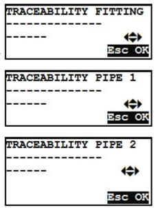
When all the traceability input data has been completed, the MSA displays a summary of the fusion parameters.
