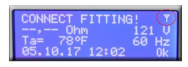
appear in the upper right hand corner of the display. When the icon is present, the GPS coordinates for each individual fusion are stored in the fusion memory. If the icon is not present, GPS signal has not yet been acquired or has been lost.
