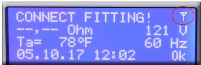
appear in the upper right hand corner of the display. When the icon is present, the GPS coordinates for each individual fusion are stored in the fusion memory. If the icon is not present, GPS signal has not yet been acquired or has been lost.
