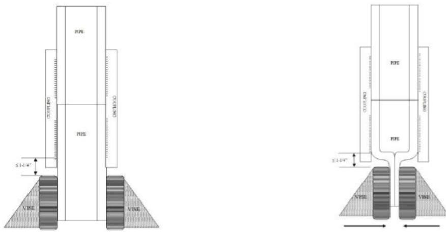
Inspect the crushed specimens for separation of the pipe and fitting in the fusion zone. Some minor separation at the fusion interface (up to 15%) may be seen at the outermost region of the fusion zone, this does not constitute failure. Ductile failure of the pipe, fitting, or PE insulation around the wires is
