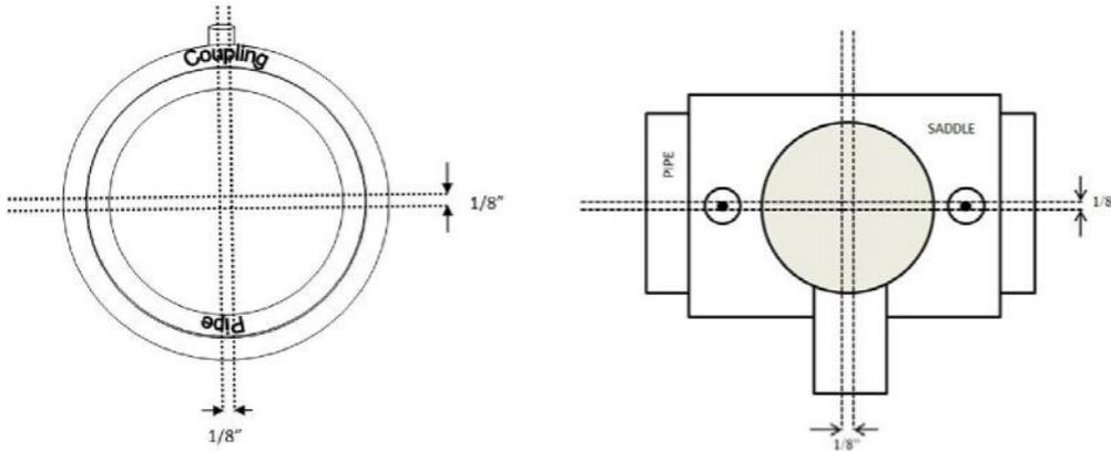
Cut FET specimens approximately  $\frac{1}{16}$  to  $\frac{1}{8}$  inches wide from each fusion or joint half. A minimum of four FET strips shall be cut from each end of the socket and from the saddle spaced approximately  $90^\circ$  apart.
