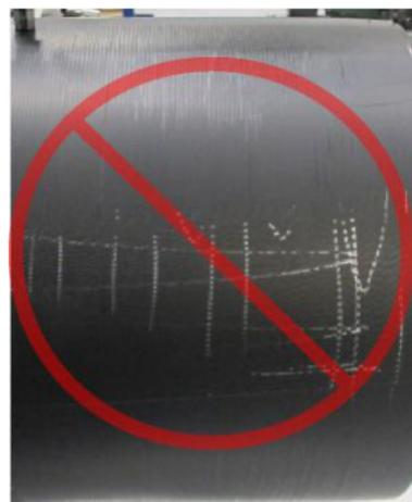
Poor scrape: markings not removed
