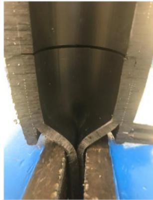
Coupling Crush Test: PASSING
