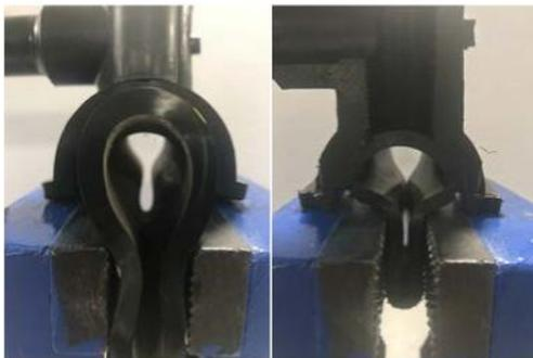
Saddle Crush Test: PASSING
