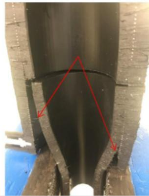
Coupling Crush Test: FAILURE
