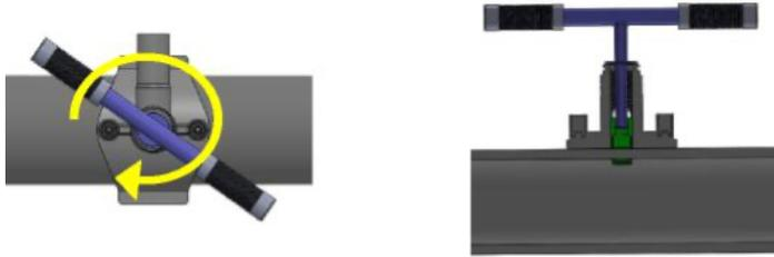
4. Back punch upward by rotating counter-clockwise until the punch is flush with the top of the fitting chimney. **STOP! DO NOT REMOVE PUNCH FROM CHIMNEY!**
