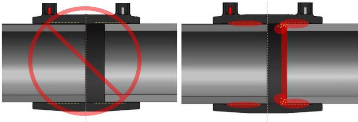
**Mis-Stab** – Incorrect Assembly: A mis-stab is another avoidable assembly error where the pipes are not located in the center cold zone of the coupling. In this case, one pipe end is over-inserted into the coupling, while the other is under-inserted. Melt again is allowed to escape between the pipe ends and the potential for heating coil shorting is likely.
