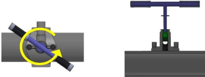
5. Remove tapping tool. Lubricate cap and chimney O-rings if needed and replace cap. Tighten cap hand tight only, do not use wrenches. Check for leaks per normal procedures.
