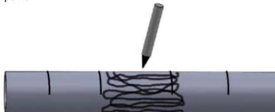
3. Scrape/peel the pipe to remove the surface layer and expose clean virgin pipe beneath. Inspect the scraped/peeled pipe surface thoroughly to ensure that all marks are removed and that only virgin pipe surface is exposed.
