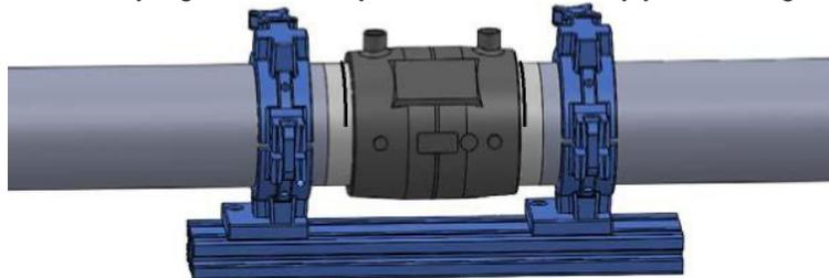
10. **Connect the control box leads to the fitting**, verify proper fusion time and voltage is displayed by the control box, and fuse the joint. Do not leave a fusion unattended.
