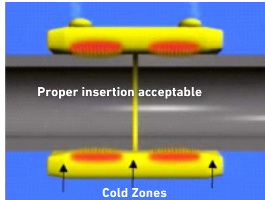
A pipe end that is not inserted beyond the innermost heating wire is commonly referred to as being “short-stabbed” and is the result of an assembly error.
