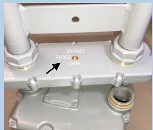
5 Turn the Co-Pilot to PURGE. Purge for one revolution of 1/2 ft mark.
