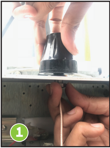
Remove the existing 3G antenna
