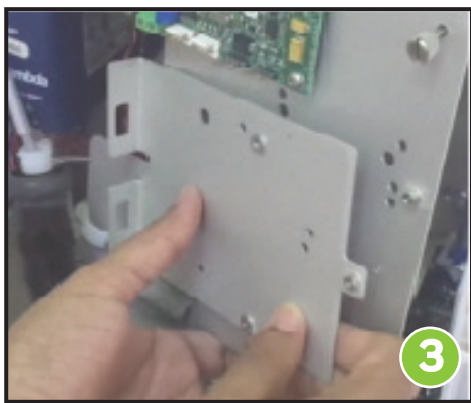
Screw the mounting bracket onto the Pivot/Sub panel to hold the Modem
