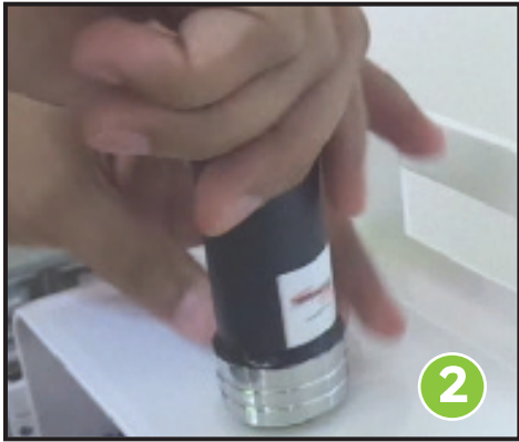
Install the 4G antenna on the MiWireless device by tightening the nut
