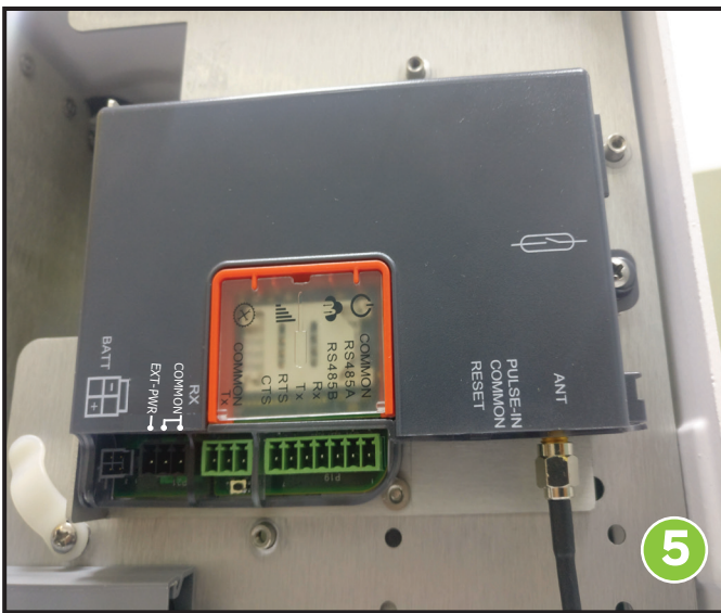
Connect the CloudLink 4G M1Modem antenna using a wrench with torque 4-6 IN-LB
