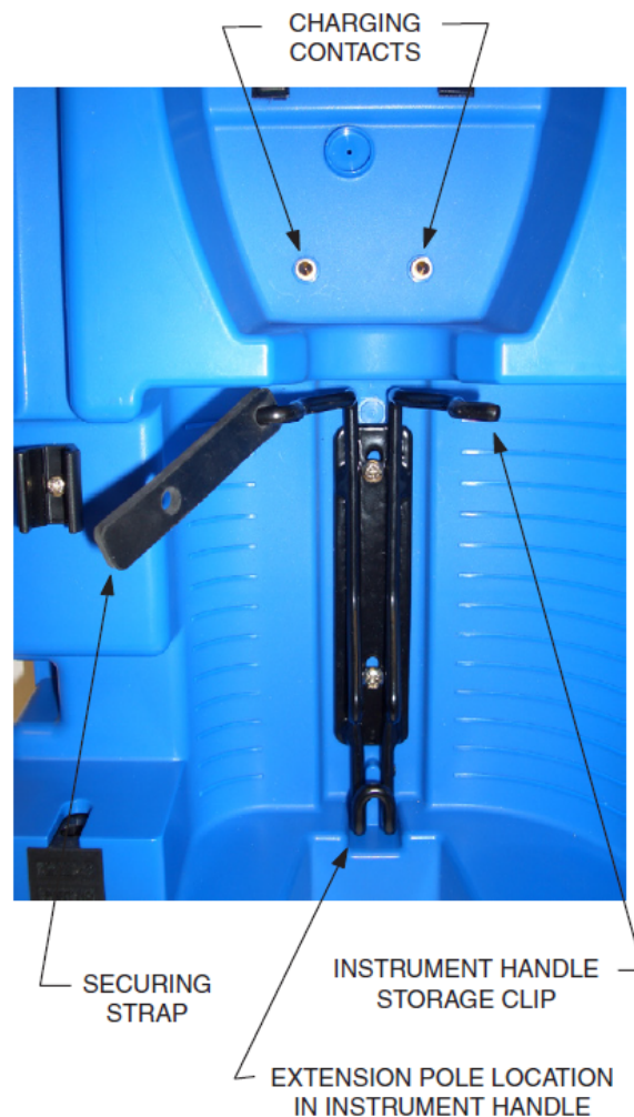
Figure 62: Charging Station - Monitor Location
