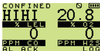
Figure 21: Confined Space Display (in alarm)
