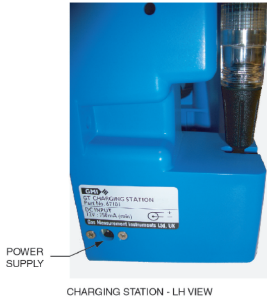
Figure 63: Power Supply to Charging Station
