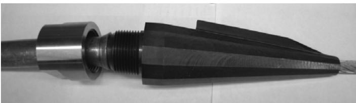
**“The Wedge SE” shown ready to install cooper pipe using the compression connector provided by Footage.**
