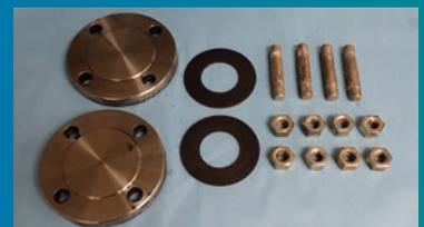
End result: Flange, nuts and bolts badly corroded making flange seal failure possible and maintenance difficult at best.
